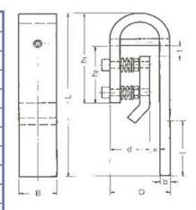
The ERKO® contact head FK is pushed onto the work or cathode rail from the top downwards. A flexible clamping plate presses the work rail against the contact surface of the head. The contact
