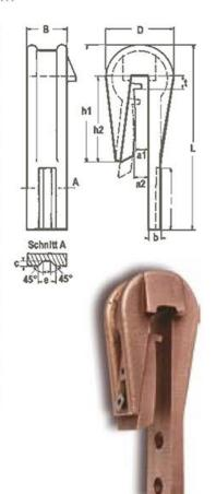
The ERKO® contact head is pushed onto the work or cathode rail from the top downwards. A clamping plate presses the contact surface of the head, via the wedge effect of the slideway guide, against the work rail, and thus establishes the non-positive contacting. The wedging can be easily released, either by the manual lever, which is pushed between the work rail and a lug provided on the contact head, or by with counter
